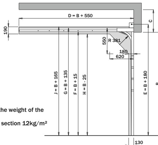
**EN** A - opening width max. 6 000mm (from door width 4 751mm there is necessary to add the weight of the struts, number of struts equals the number of the sections, strut weight 1,25 kg/lm)
